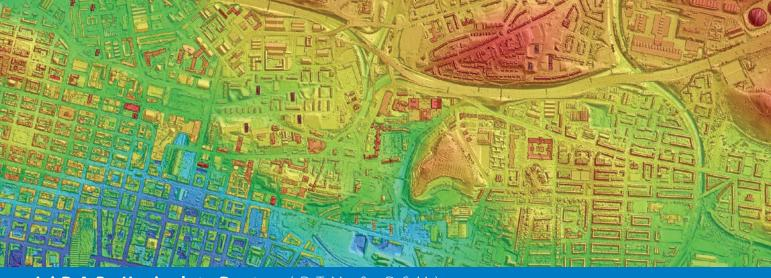
LiDAR Height Data (DTM & DSM)
