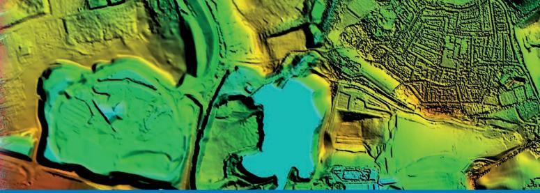
Digital Terrain Model (DTM) Digital Surface Model (DSM)
